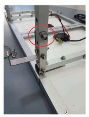
6. Put the bold and nut back in the marked hole and screw tight. Do this for both brackets.
