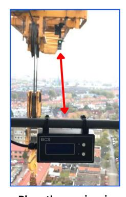
Place the receiver in line of sight with the camera as good as possible.
